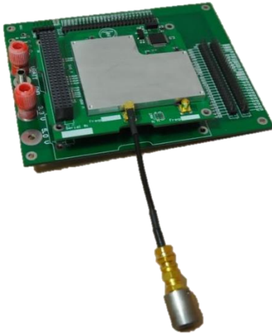
Figure 2 – He-100 with 50 Ohm load attached
