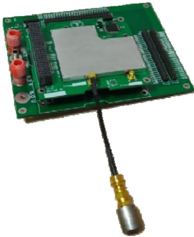
Figure 2 – He-100 with 50 Ohm load attached
